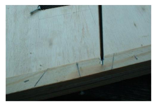
Now insert the woodscrews after countersinking the hole with the screwdriver bit to make sure the head sits flush.  $\,$
