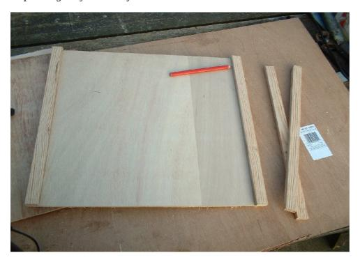
Now we need to glue and staple or pin the edges on to both sides of the board. Its very important that we don't glue or pin the middle 150mm of each edge because we want a pivoting door here
