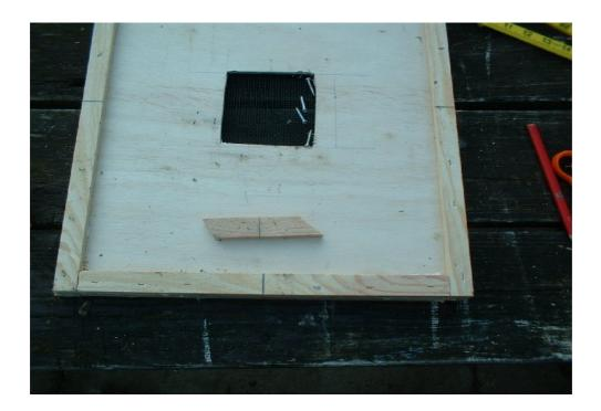
Now mark the centre of each edge and make a template for your doors from a scrap of strip wood. The template needs to be around 100mm long with a sloping cut front and rear edge approx 45° Mark the centre of the template as shown
